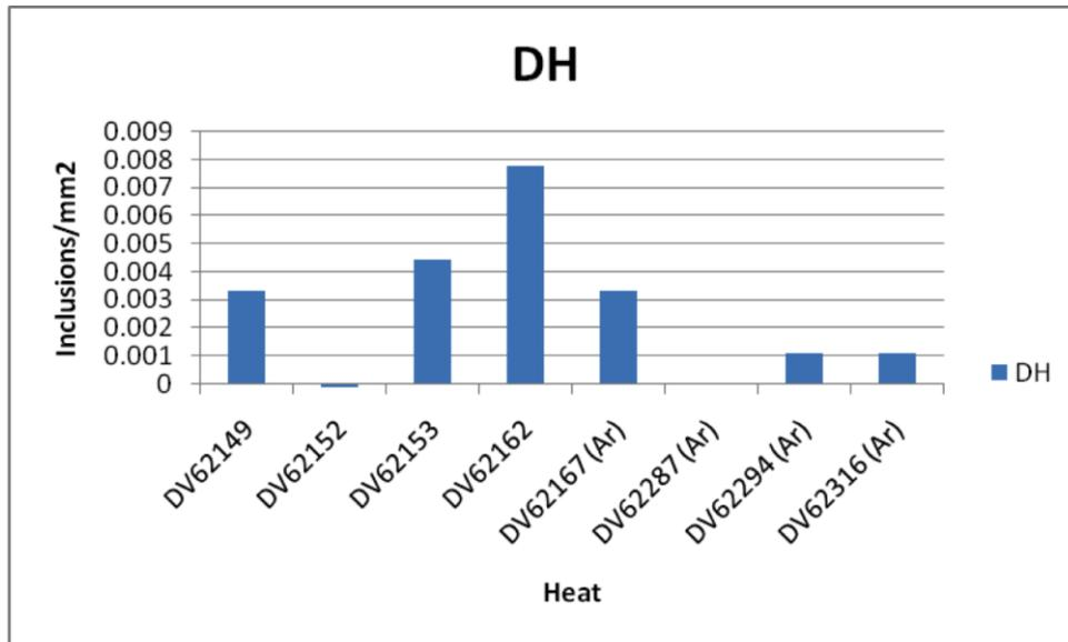
**Figure 29:** Amount of removed DH type inclusions/mm<sup>2</sup> during the final stirring period.
