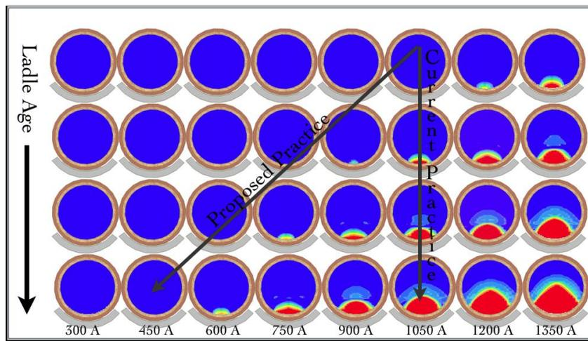
**Figure 10:** Open eye size as a function of ladle wear and stirring current
