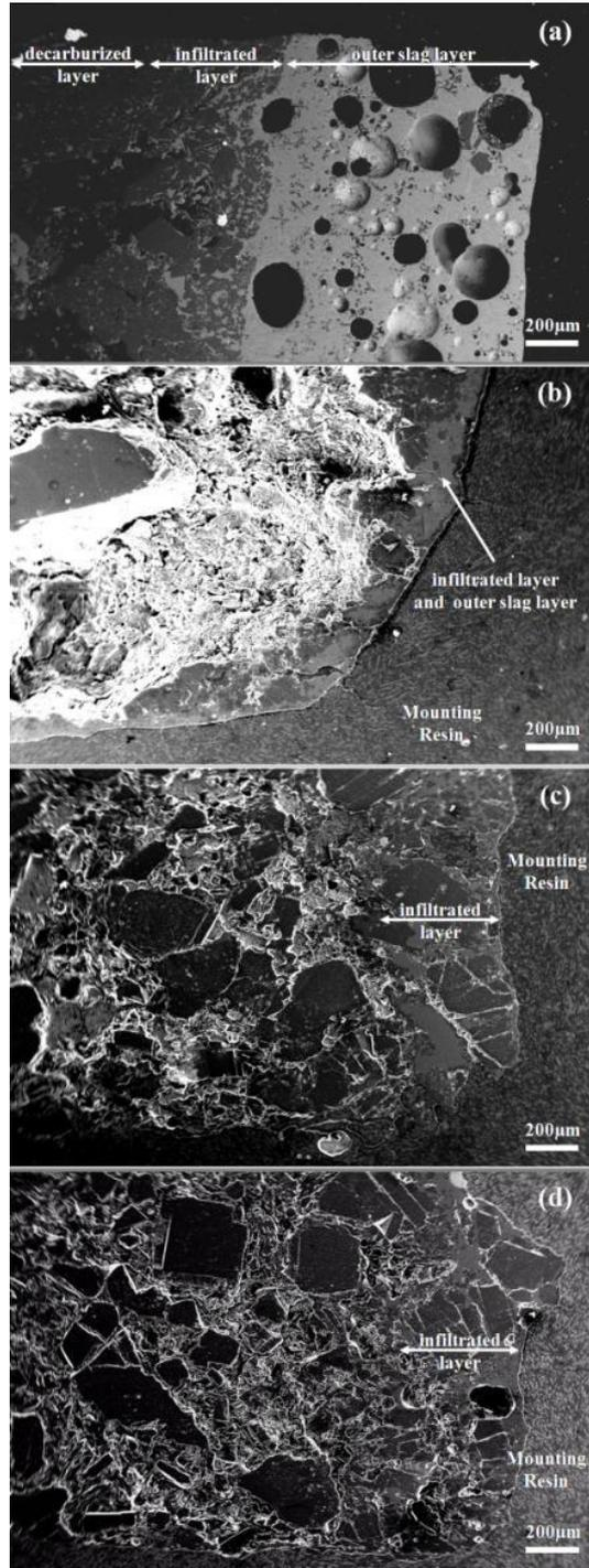
**Figure 23:** SEM pictures of glazed refractory samples (a. Before experiment, b. After experiment (5 min.), c. After experiment (120 min.), d. After experiment (rotated in steel))
