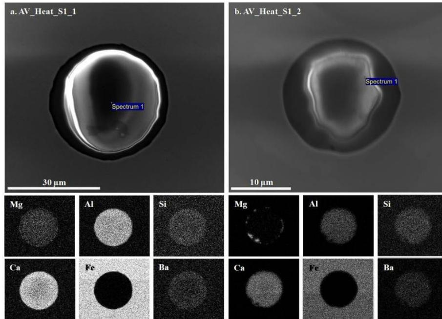
**Figure 20:** The SEM micrograph and element mappings of type 7 inclusions
