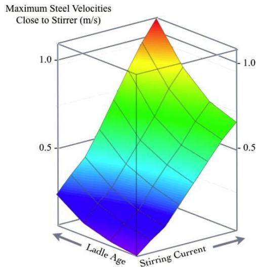
**Figure 9:** Maximum steel velocities in the ladle as a function of ladle age and stirring intensity.
