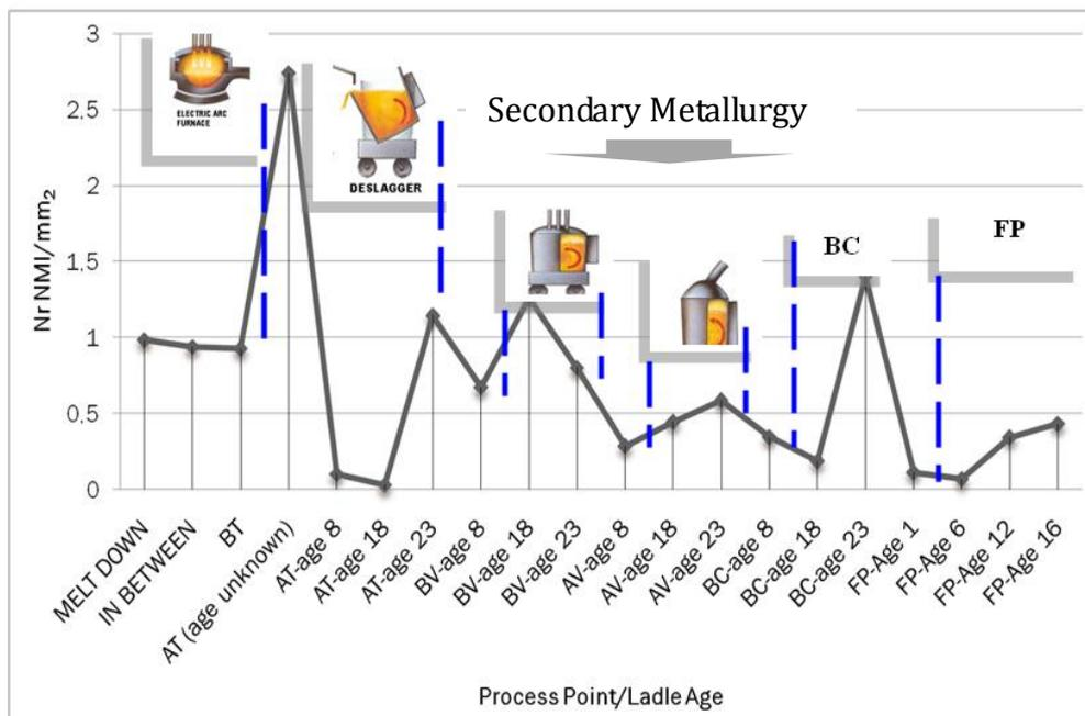
**Figure 31:** Evolution of NMI during different production steps at Uddeholm, where MD is Melt down, IN BETWEEN during treatment in the EAF, BT and AT stands for Before tap and after tapping of the EAF, BV: Before vacuum, AV: After vacuum, BC: Before casting and FP: End product. The numbers refer to the ladle age.
