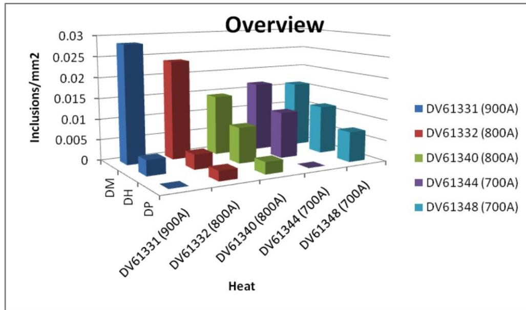
**Figure 27:** The amount of removed inclusions /mm<sup>2</sup> during the vacuum treatment (trials 1-5)
