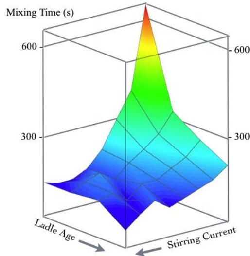
**Figure 11:** Mixing times for induction stirring as a function of ladle age and stirring current.
