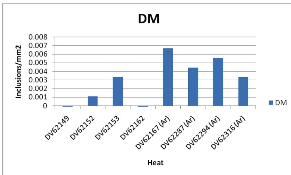
**Figure 28:** Amount of removed DM type inclusions/mm<sup>2</sup> during the final stirring period.
