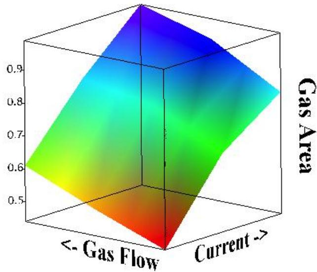
**Figure 8:** Gas plume area as a function of induction stirring current and gas flow rate
