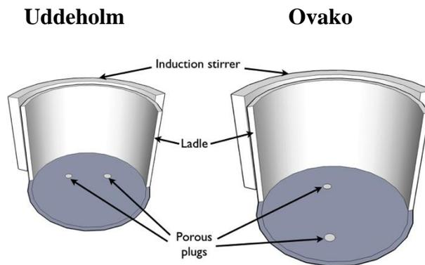
**Figure 4:** Placement of induction stirrer and porous plugs at Uddeholm and Ovako.
