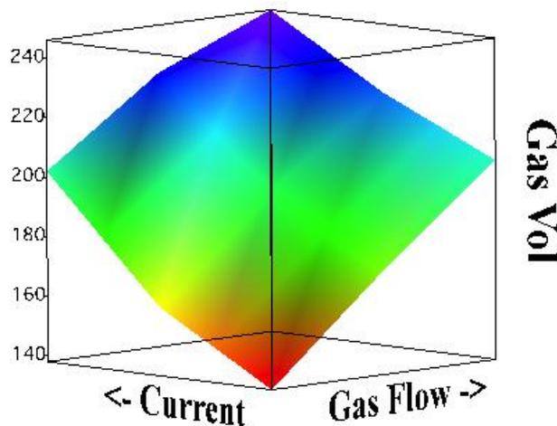
**Figure 7:** Gas volume in steel as a function of induction stirring current and gas flow rate.
