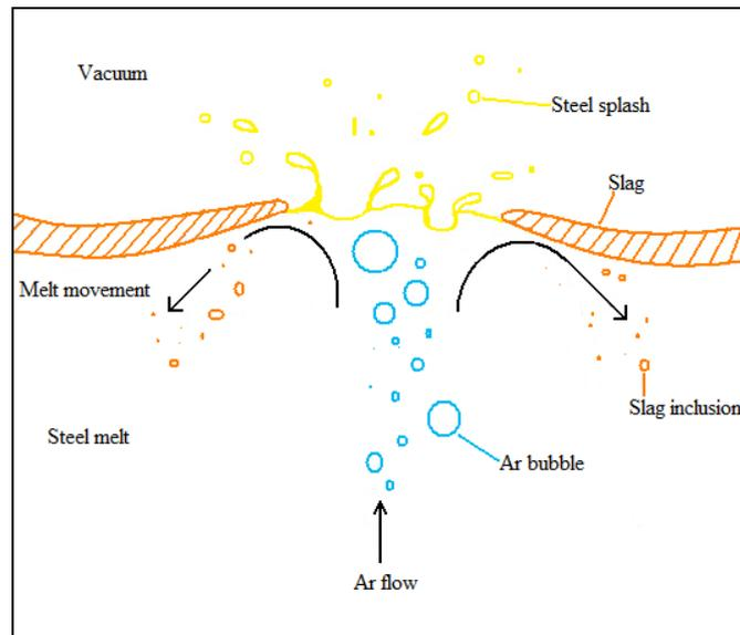
**Figure 3:** Schematic illustration of slag/metal movement close to the open eye during vacuum treatment with argon stirring
