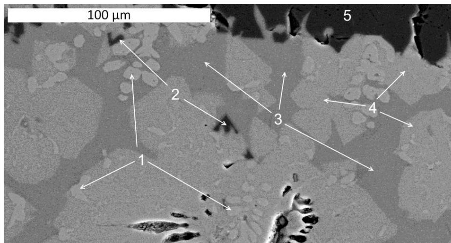
**Figure 21:** SEM microphotograph of sample R2; 2CaO.SiO<sub>2</sub> marked as 1, MgO marked as 2, super cooled liquid marked as 3, 3CaO.Al<sub>2</sub>O<sub>3</sub> as 4, and the MgO rod is marked as 5.
