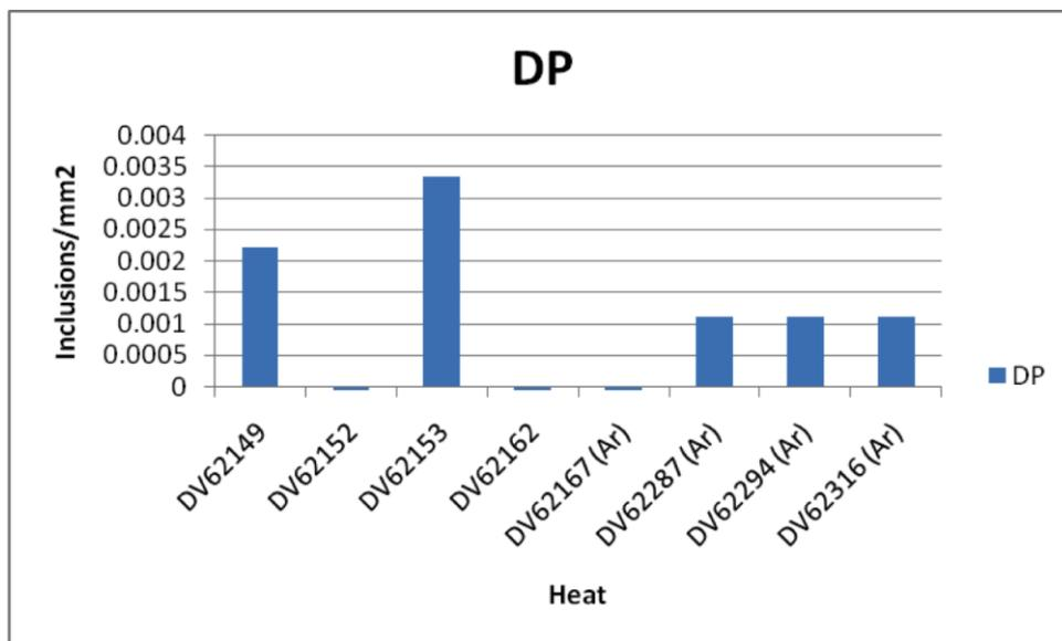
**Figure 30:** Amount of removed DP type inclusions / mm<sup>2</sup> during the final stirring period.
