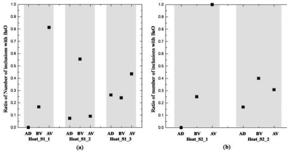
**Figure 19:** Fractions of the number of inclusions with BaO at various process steps (a. Heat series 1, b. Heat series 2)
