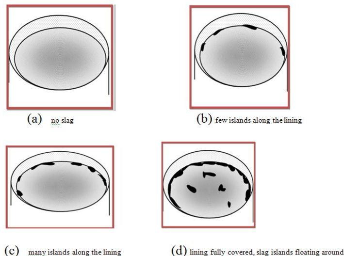
**Figure 25:** 4 scales of estimating amount of carry-over slag were used to monitor the efficiency of the deslagging process.
