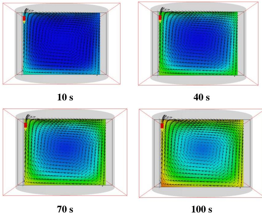
**Figure 12:** Generation and separation of inclusions from the ladle wall as a function of stirring time.
