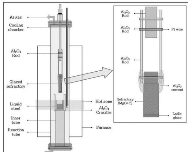
**Figure 2:** Experimental setup for steel-glaze reaction study
