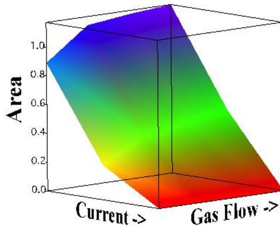
**Figure 6:** Area of open eye as a function of induction stirring current and gas flow rate.
