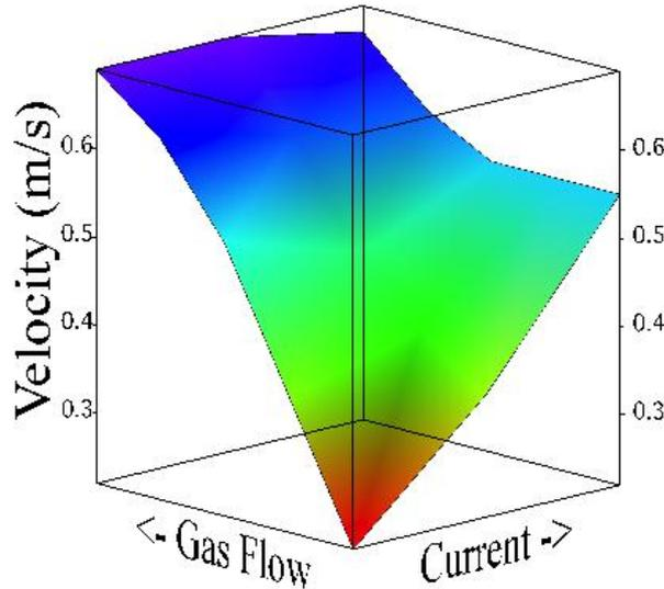
**Figure 5:** Maximum steel velocities in the ladle as a function of induction stirring current and gas flow rate.
