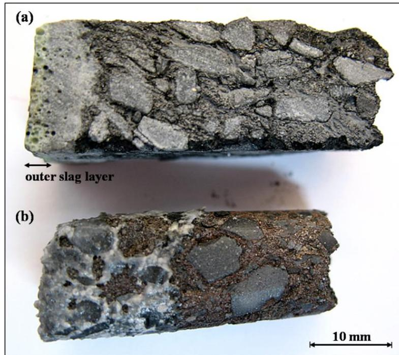
**Figure 22:** Comparison of the glazed refractory samples before and after experiments
