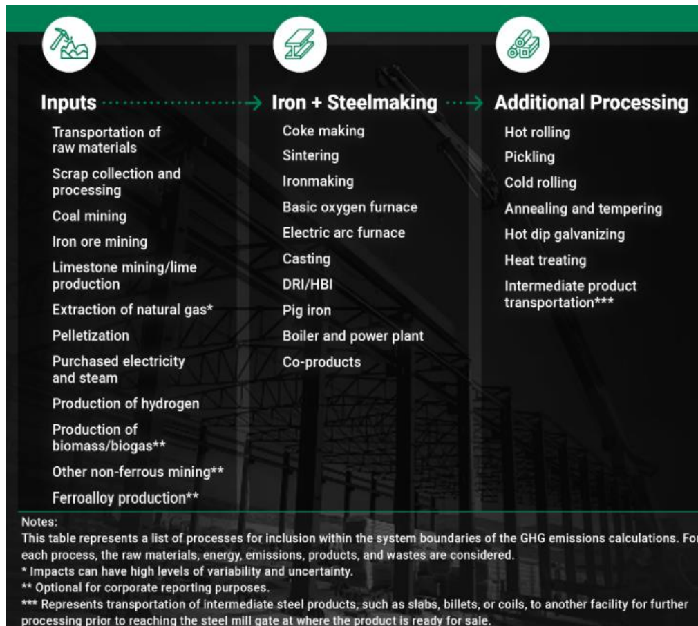
Figure A2- 10 Recommended System boundaries for consistent GHG Reporting in the Steel Industry (AISI)
