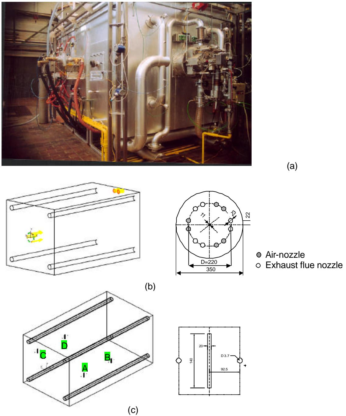
Figure 2 HiTAC test furnace and burner
