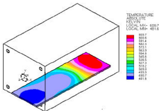
Figure 9 Predicted of temperature distribution on moving slab at one-flame HRS
