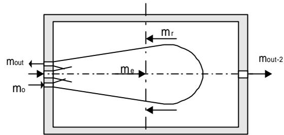
Figure 15 Scheme of structure of the flame zone and recirculation in an enclosed combustion chamber
