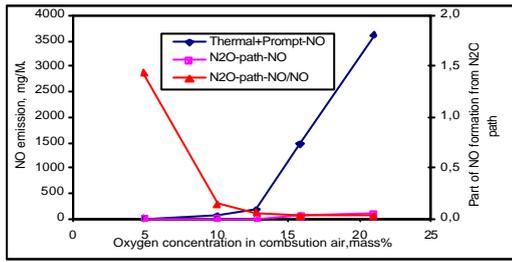
Figure 10 Effect of oxygen concentration on NO emission at air temperature of 1173K and fuel temperature of 299K for single gas jet at co-flow test
