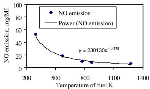
Figure 13 Effect of fuel temperature on NO emission at Stagger Mode
