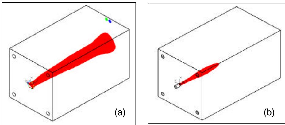
Figure 6 Predicted flame shape for HiTAC and Conventional burner
