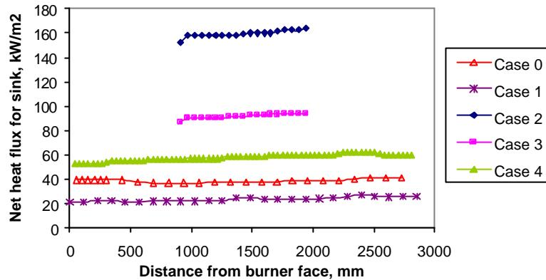
Figure 8 Predications of heat flux absorbed by the charge in test furnace
