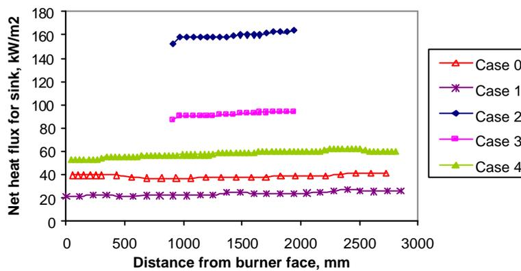
Figure 8 Predictions of heat flux absorbed by the charge in test furnace
