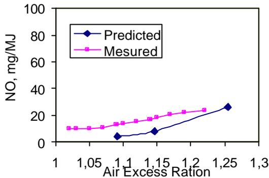
Figure 12 NO emission vs. excess air ratio at HiTAC furnace with one-flame HRS
