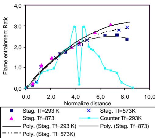
Figure 14 Effect of fuel temperature on flame entrainment ratio
