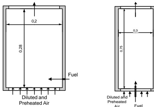
Figure1 Schematic of combustion chamber for single fuel jet test furnace
