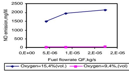
Figure 11 Effect of fuel flowrate on NO emission at single gas jet at co-flow test
