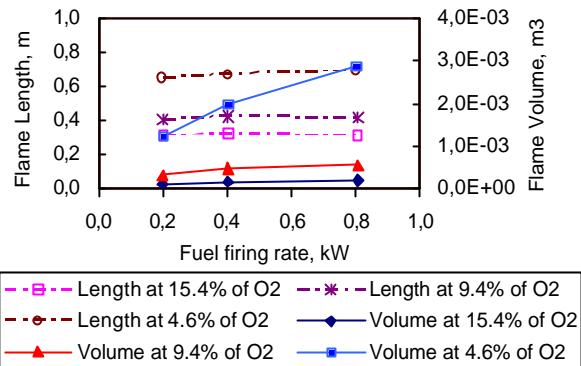
Figure 4 Flame length and volume of LPG flame at difference fuel firing rate for single gas jet with co-flow test
