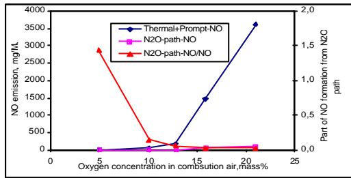
Figure 10 Effect of oxygen concentration on NO emission at air temperature of 1173K and fuel temperature of 299K for single gas jet at co-flow test
