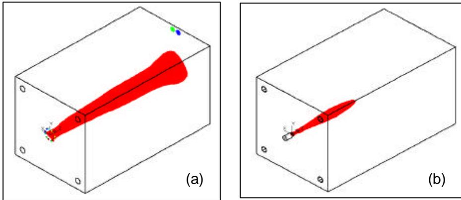
Figure 6 Predicted flame shape for HiTAC and Conventional burner
