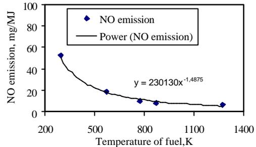
Figure 13 Effect of fuel temperature on NO emission at Stagger Mode
