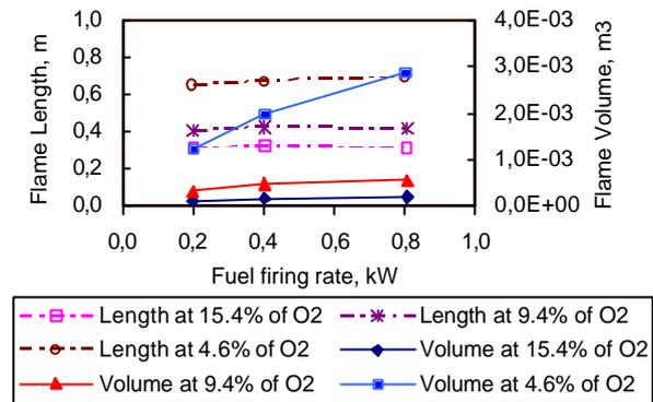
Figure 4 Flame length and volume of LPG flame at difference fuel firing rate for single gas jet with co-flow test
