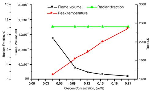
Fig.3 Flame volume, peak temperature and radiant fraction versus oxygen concentration during 1173K of air temperature and 299 K of fuel temperatures for single gas jet with co-flow test
