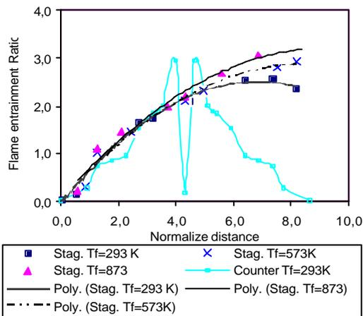
Figure 14 Effect of fuel temperature on flame entrainment ratio
