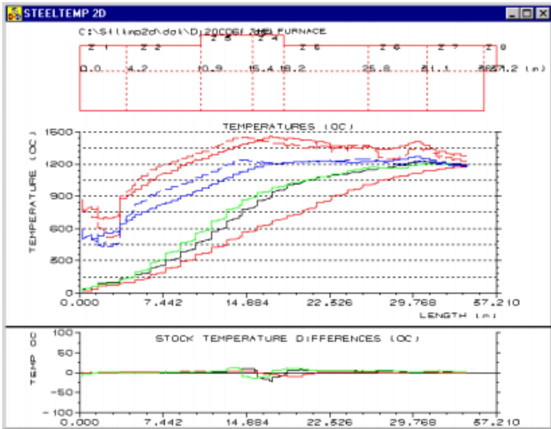
Figure 12. Gas and stock temperatures in the Steeltemp model of Furnace 302 at SSAB.
