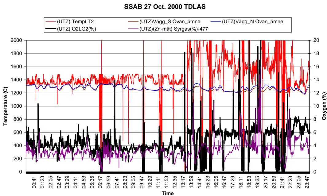
Figure 8. Instability in the simultaneous measurement of the excess oxygen and temperature in the soaking zone of SSAB Furnace 302 at low levels of excess oxygen.
