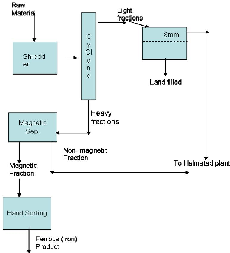
Fig.14- General configuration for Huddinge shredding and separating plant
