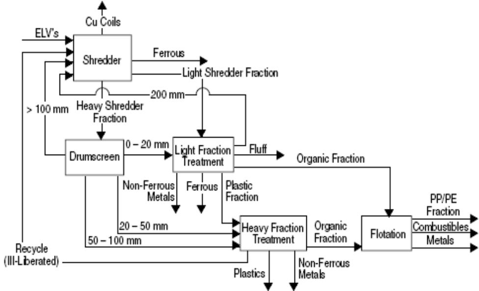
Fig.19- Simplified industrial recycling plant for ELVs due to current technology
