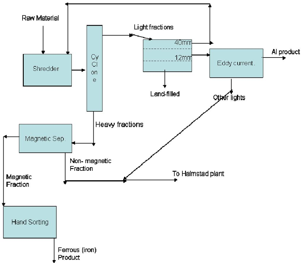
Fig.13- General configuration for Hallstahammar shredding and separating plant
