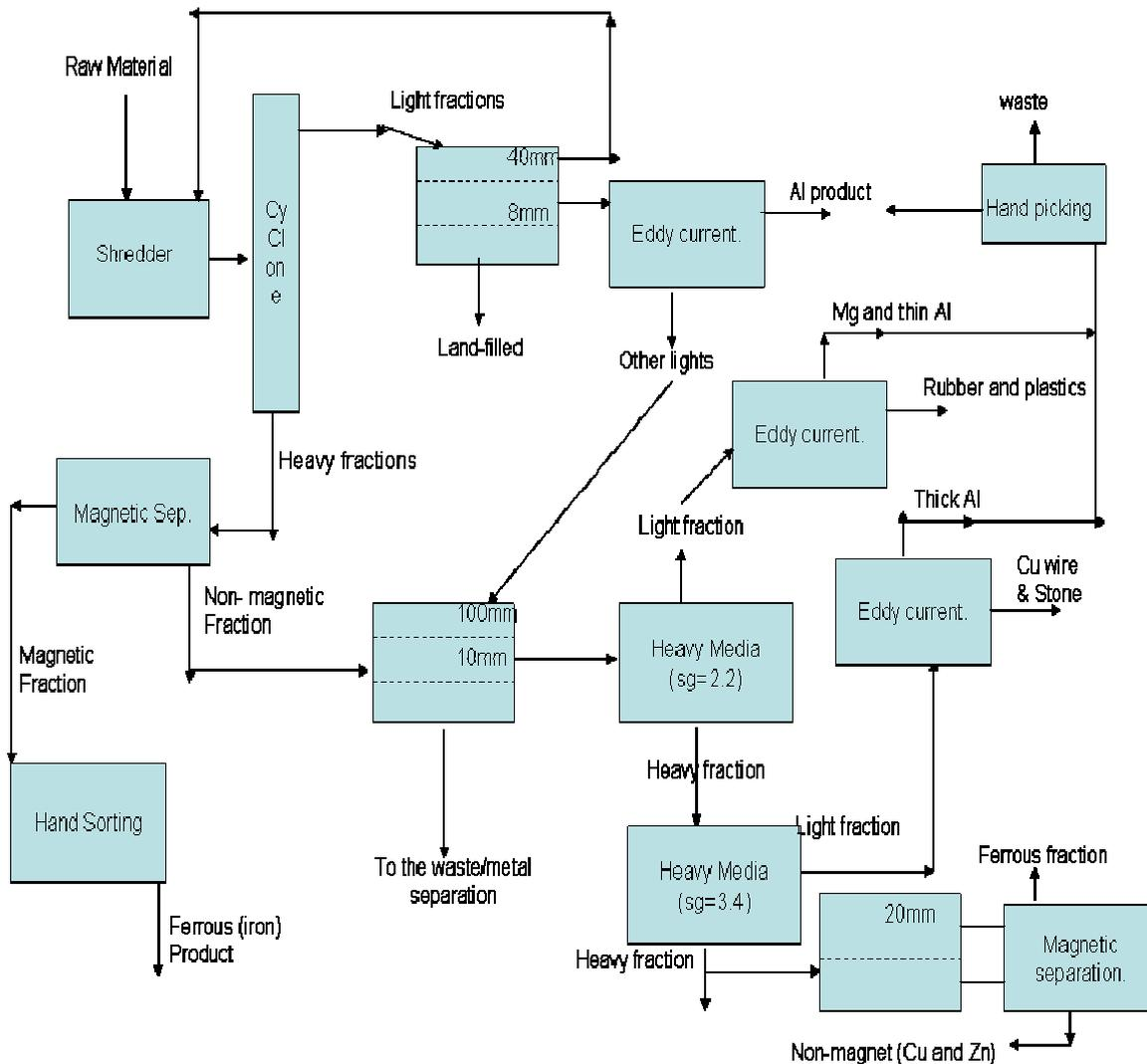
Fig.12- General configuration for current Halmstad shredding and separating plant
