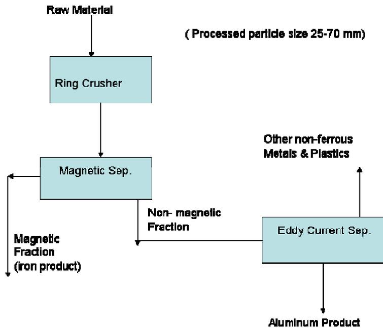
Fig.16- Kuusakoski's facility for processing electronic scrap
