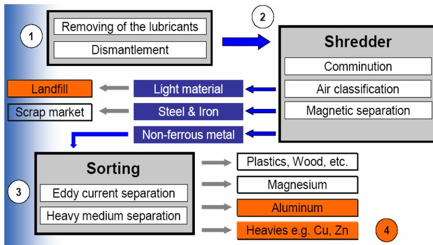
Fig.7- Schema of processes at a typical shredding facility
