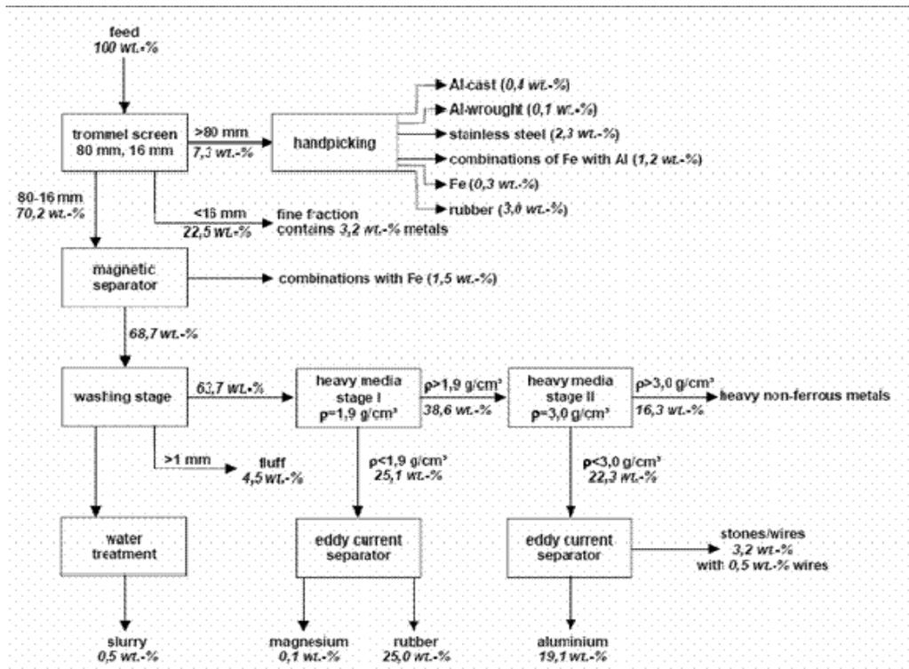
Fig.10 – General configuration for heavy media plant to separate aluminium and other metals
