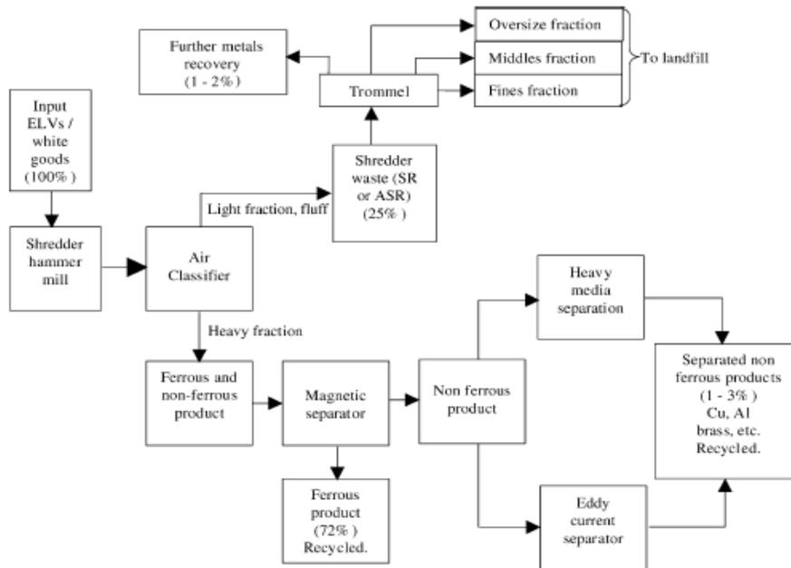
Fig.9- Configuration for recycling of ELVs
