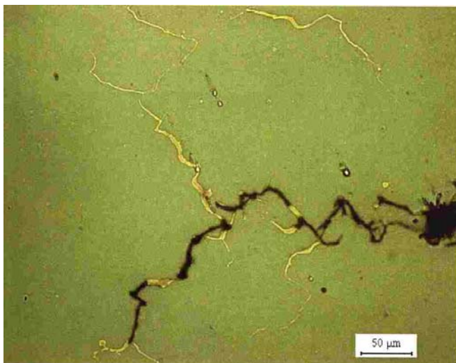
Figure 8 Cracks following austenite grain boundaries that has been infiltrated by liquid copper in a 2.5 w% Cu steel.
