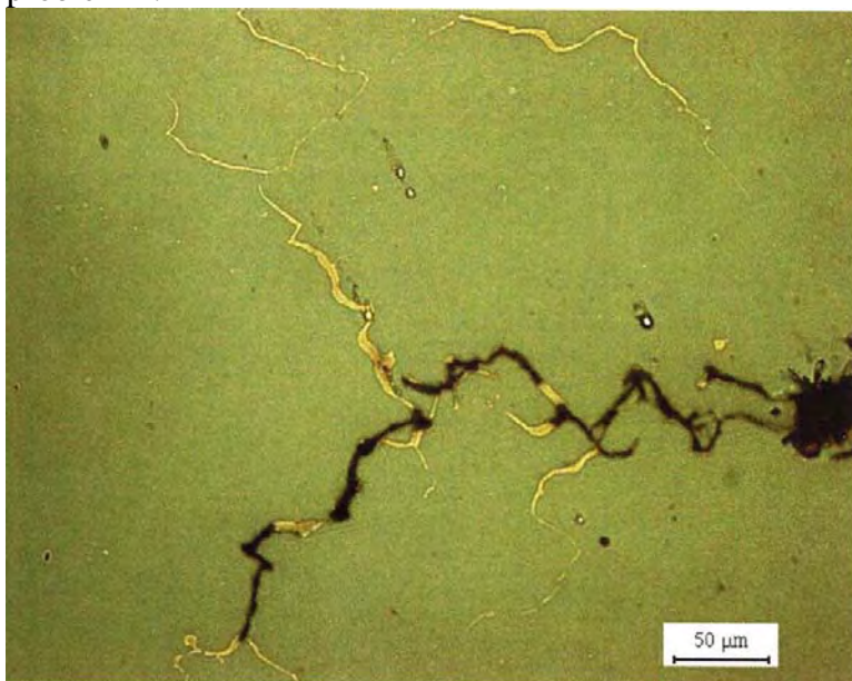
Figure 3 Cracks following austenite grain boundaries that has been infiltrated by liquid copper in a steel alloyed with 2.5 w% Cu [9] .
