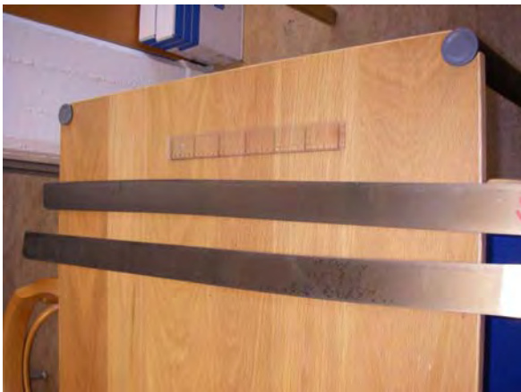
Figure 15: The material after cold rolling.
