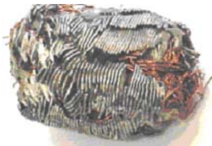
coil of electric motor containing cast iron and copper
