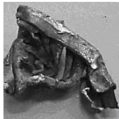
particle of aluminum with rubber insert
