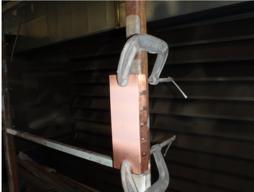
Figure 2. Set-up of the sample to be sprayed.
