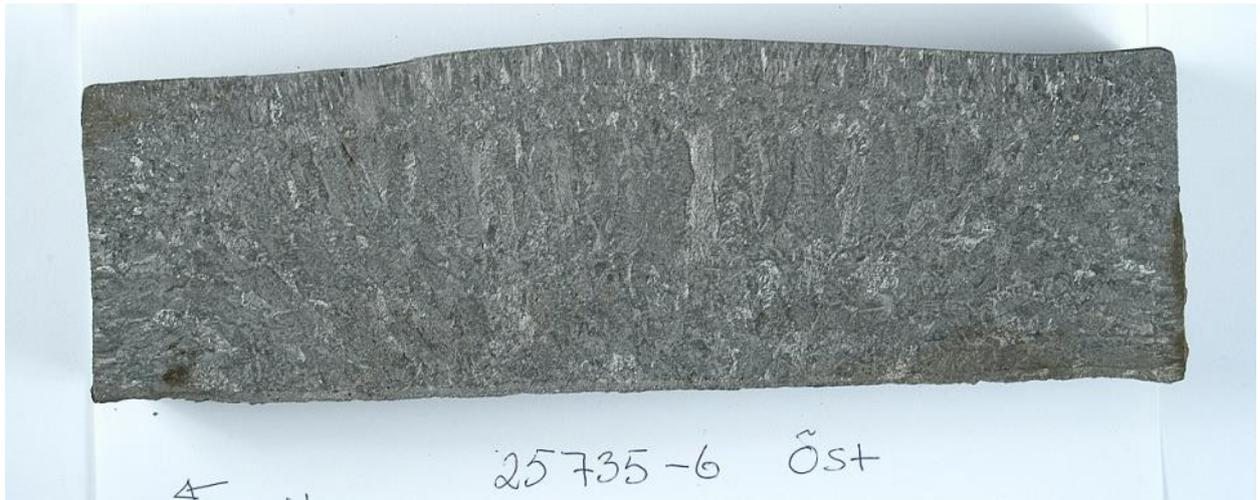
**Figure 77.** Full size picture of the etched east near narrow side transverse slab sample (arrow points to lower-fixed south side).
