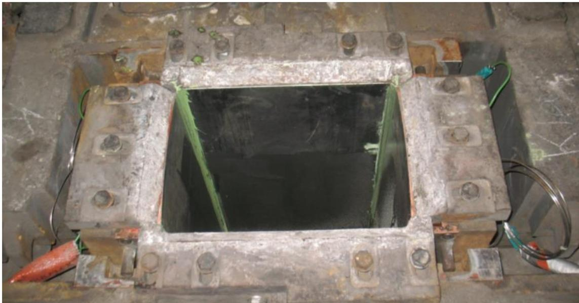
**Figure 50.** T.C. installation in the mould.
