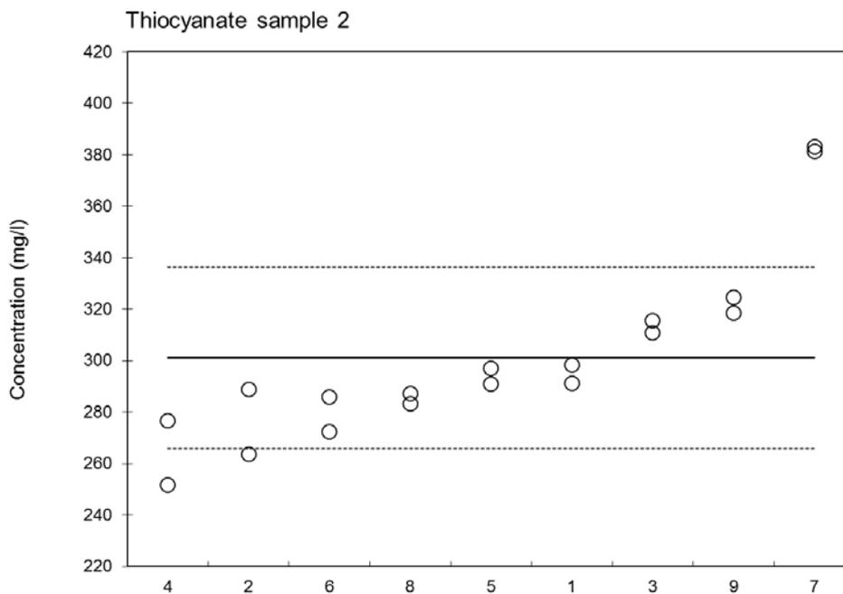
In the graph colored values indicate that the testing machine is a statistical outlier; red – Cochran outlier, blue – Grubbs single outlier, green – Grubbs by pair outliers. Straight line indicate mean value and broken lines  $\pm 1 \sigma$ .
