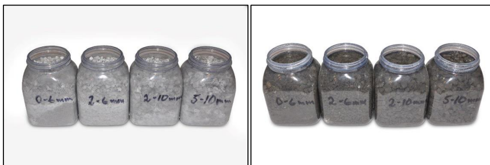
Figure 15. Color of slag that had been regularly wet and dry (left pic.) and slag that constantly had been held in water (right pic.).
