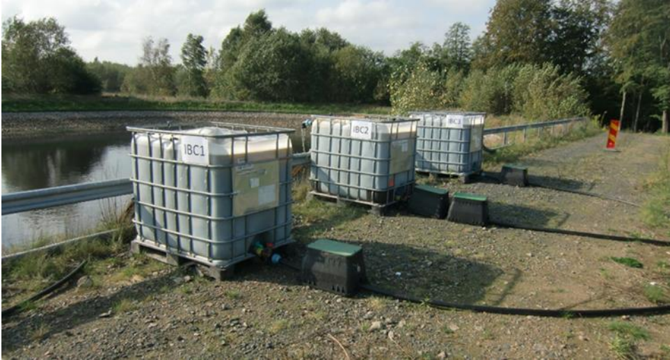
Figure 10. Experiment with treatment of landfill leachate in IBC-containers filled with Petrit E.
