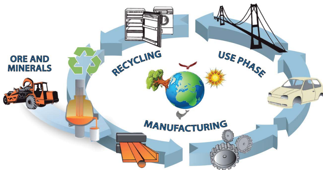
Figure 1.1 Life Cycle Assessments reflect a product's overall material and energy flows as well as the emissions to air, land and water, all from a life cycle perspective.
