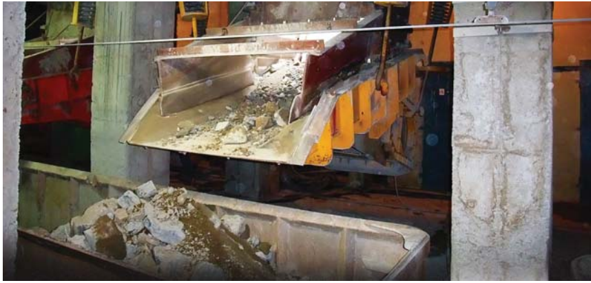
Figure 3.12 Example of a chute used in mines; its life span can change through the use of harder steel.
