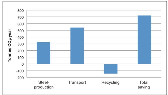
Reduced greenhouse gas emissions from steel production and transportation of high strength steel chair frames when compared with chair frames in conventional steel.
